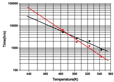
Thermal Endurance has been carried out on Helical Coils to ASTM D3145 and **Twisted Pairs** to ASTM D3251 (as recognised by Underwriters Laboratories).
